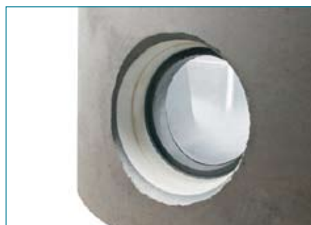
Fig. 8 Connections: pipe connections according to customer request. Separate channel lining is not necessary. The socket is shaped during the concreting process.
