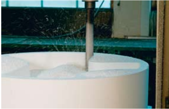
Fig. 4 Production of the channel negative by the BFS block milling machine.
