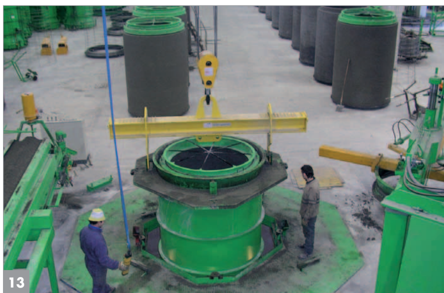
The oscillating pressed steel spigot forming ring is maintained on the top of the product until the end of the curing phase
