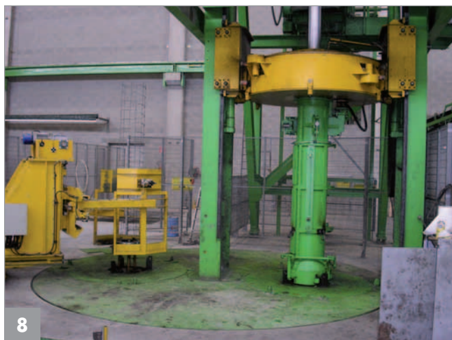
Cart for reinforcement cages
