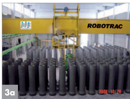
Demoulding area for the pipes
