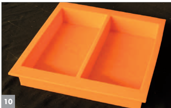
Double-mould for half-sized elements
