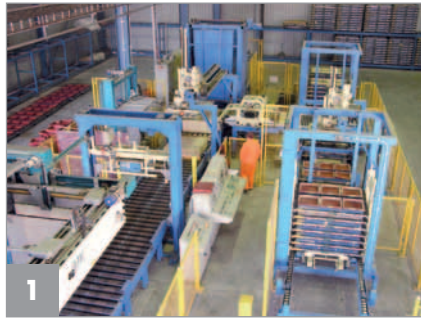
The plant, which is divided into separate lines for wet and dry production sequences, is designed for fully automatised manufacture of concrete block and slab paving
