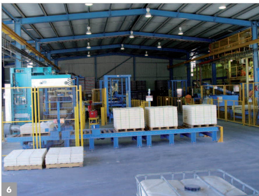
6 The completed delivery paletts are transported via a conveyor belt to the storage plant
