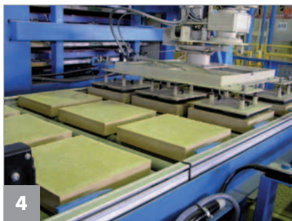
4 Stripping of the moulds is done automatically and all moulds of a palett are stripped at the same time
